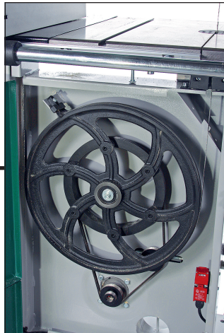
A two-step pulley on the bottom wheel controls the blade speed
