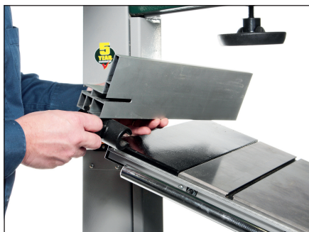
You can remove the rip fence without having to tilt the table
