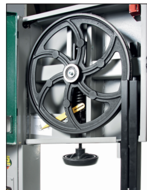
The cast iron band wheels are coupled to a robust tensioning mechanism
